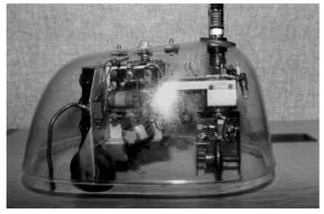
One of Walter's robots was named Machina Speculatrix ("machine that thinks"). It consisted of a photocell, a bump sensor, a rechargable battery, three motors, three wheels, and one analog circuit. It had the following capabilities:<sup>2</sup>
